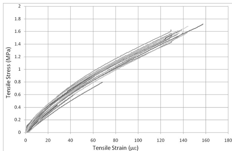
**Figure 8 - Stress-strain curves of concrete in direct uniaxial tension**
