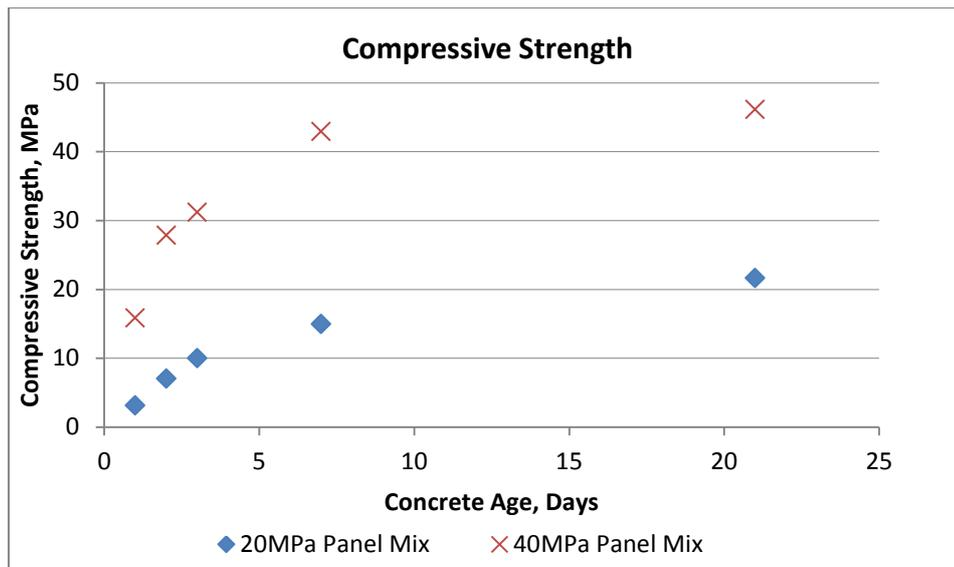
**Figure 11: Concrete compressive strengths measured for each batch**
