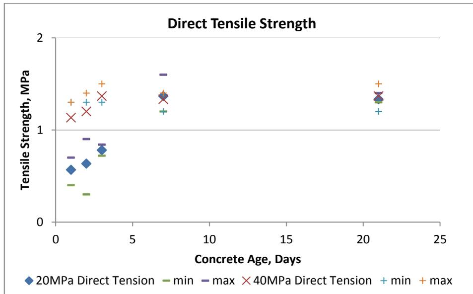
**Figure 13: Comparison of measured direct tensile strengths for both batches**
