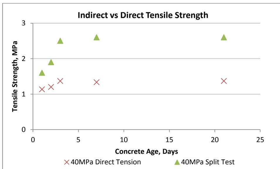
**Figure 12: Comparison of measured indirect and direct tensile strengths**
