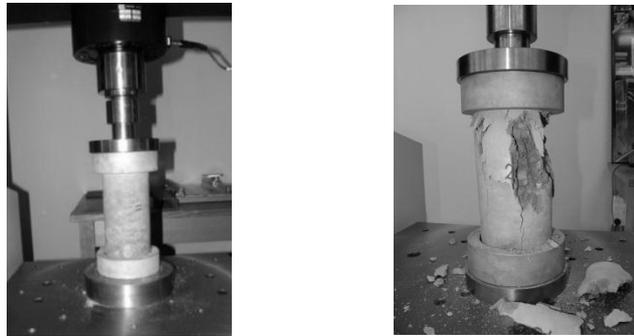
**Figure 5: Compression test setup, and a typical failure at early age (1 day)**
