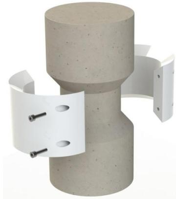
**Figure3: Direct tension test specimen**
