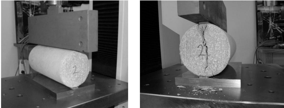
**Figure 7: Split test setup, and typical fracture.**
