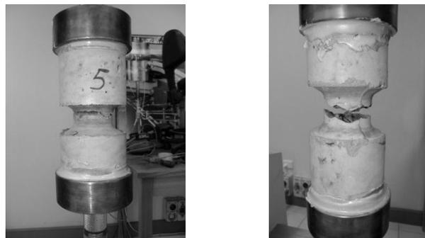
**Figure 6: Tensile test setup, and typical failures of tensile cylinder**
