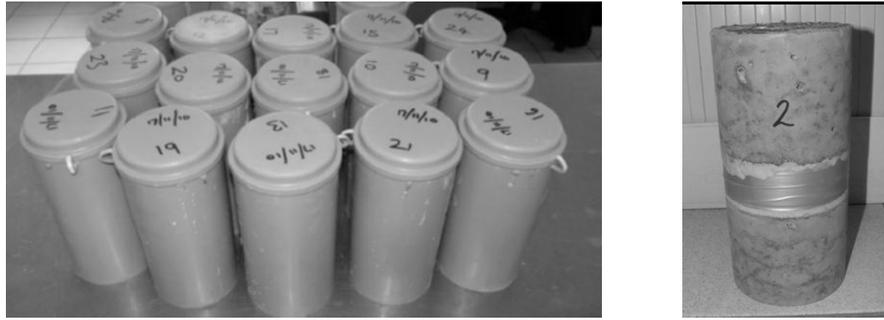
**Figure 4: Cylinder moulds, and a demoulded cylinder prior to reduced section being stripped**
