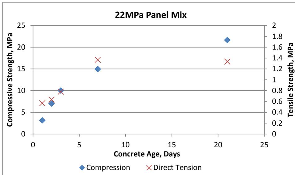
**Figure 9: Concrete strengths observed for 22MPa batch**
