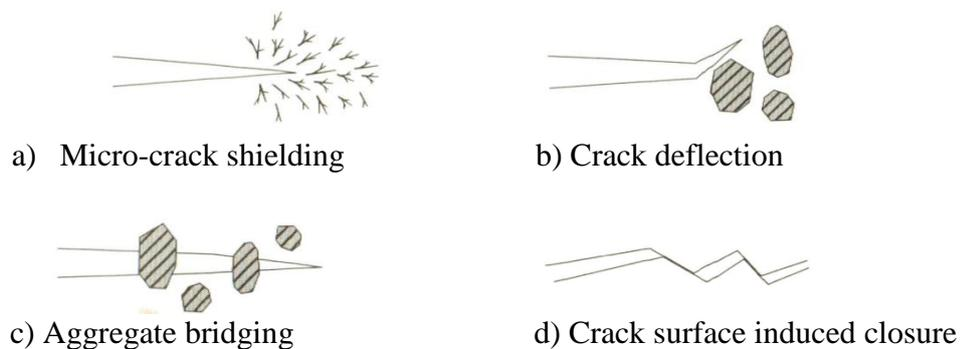
**Figure 2: Crack propagation interactions of concrete in tension**
