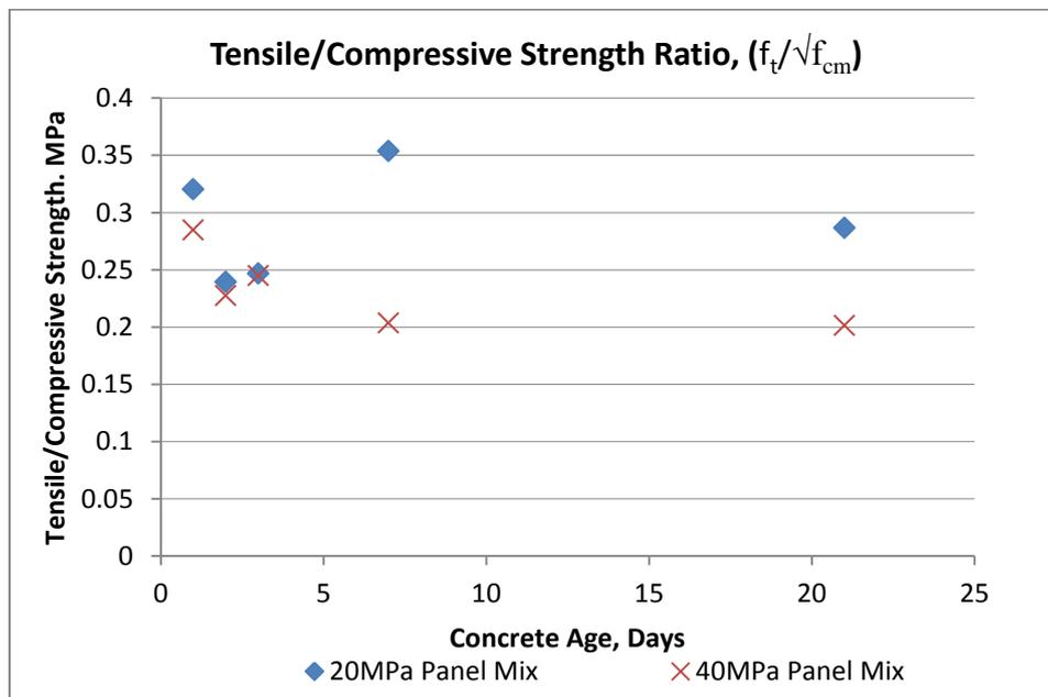
**Figure 14: Comparison of tensile/compressive ratios between both batches**
