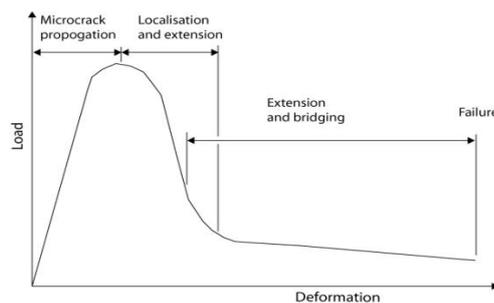
**Figure 1 - Simple schematic showing a load deformation curve of concrete in tension (Nomura [14])**
