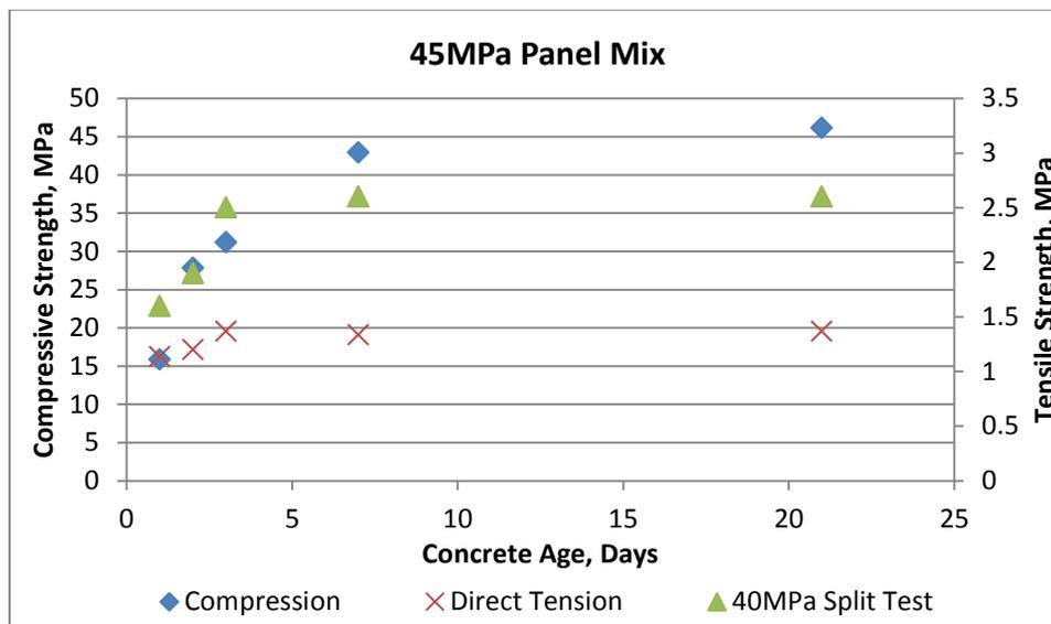
**Figure 10: Concrete strengths observed for 45MPa batch**
